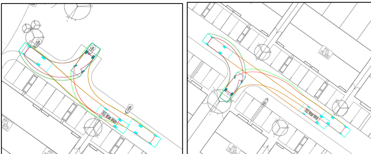
Figure 3.8.2 - Selection of turning head areas throughout the development with refuse vehicle movements autotracked to confirm accessibility (Source: ORS drawing 241139-ORS-ZZ-00-DR-TR-731)
